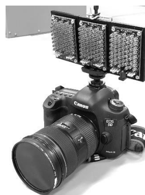
Fig.1 Modified IR Single-lens Camera with IR light projector.
