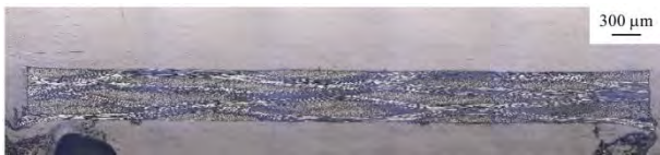
(1) SEM image of plasma-treated FRP composite.
